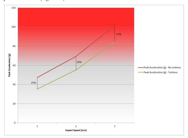
Results for the low speed linear impact tests conducted at 1 m/s, 2 m/s and 3m/s are presented below (Figure 4-4).
