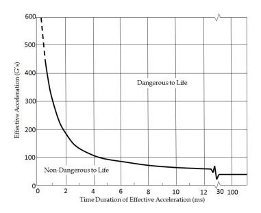
Figure 2-1: Wayne State Tolerance Curve [1]
