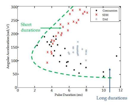
Figure 2-2: Acceleration vs. time injury tolerance curve [2]
