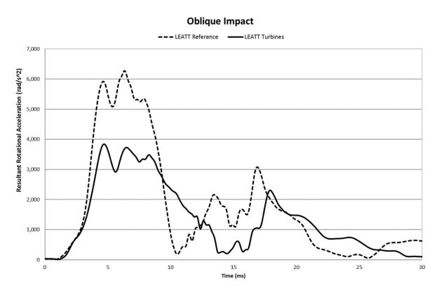
Figure 4-3: 6.1 m/s rear oblique impact - illustration of transferred energy reduction
