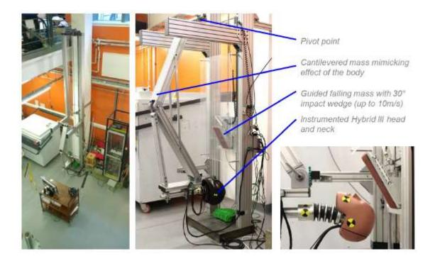
Figure 4-1: Oblique impact helmet test rig
