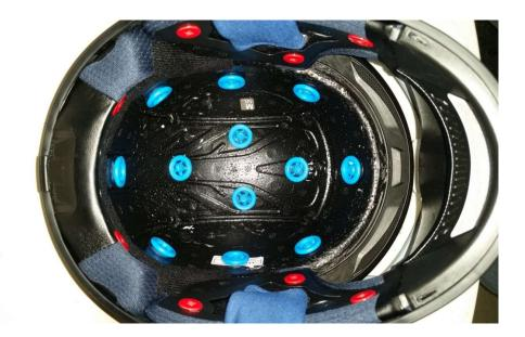
Figure 3-3: Tubines in place within the EPS structure
