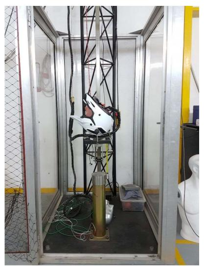
Figure 4-2: ECE 22.05 test rig
